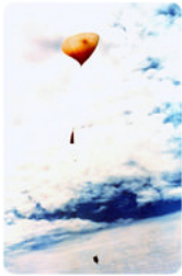
A weather balloon with a radiosonde beneath it. The radiosonde is the bottom piece and the parachute that will bring it to the ground is above it. [Figure3]
